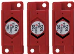
Figure 3-6 Shock indicator tripped
