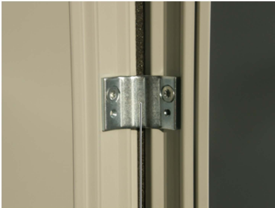
Cabinet connector, outer Tightening torque: 9 Nm
