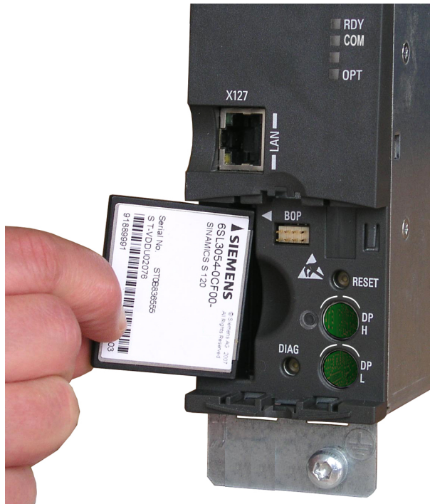
Figure 4-52 Slot for the memory card
