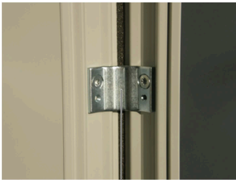
Outer cabinet connector Tightening torque: 9 Nm
