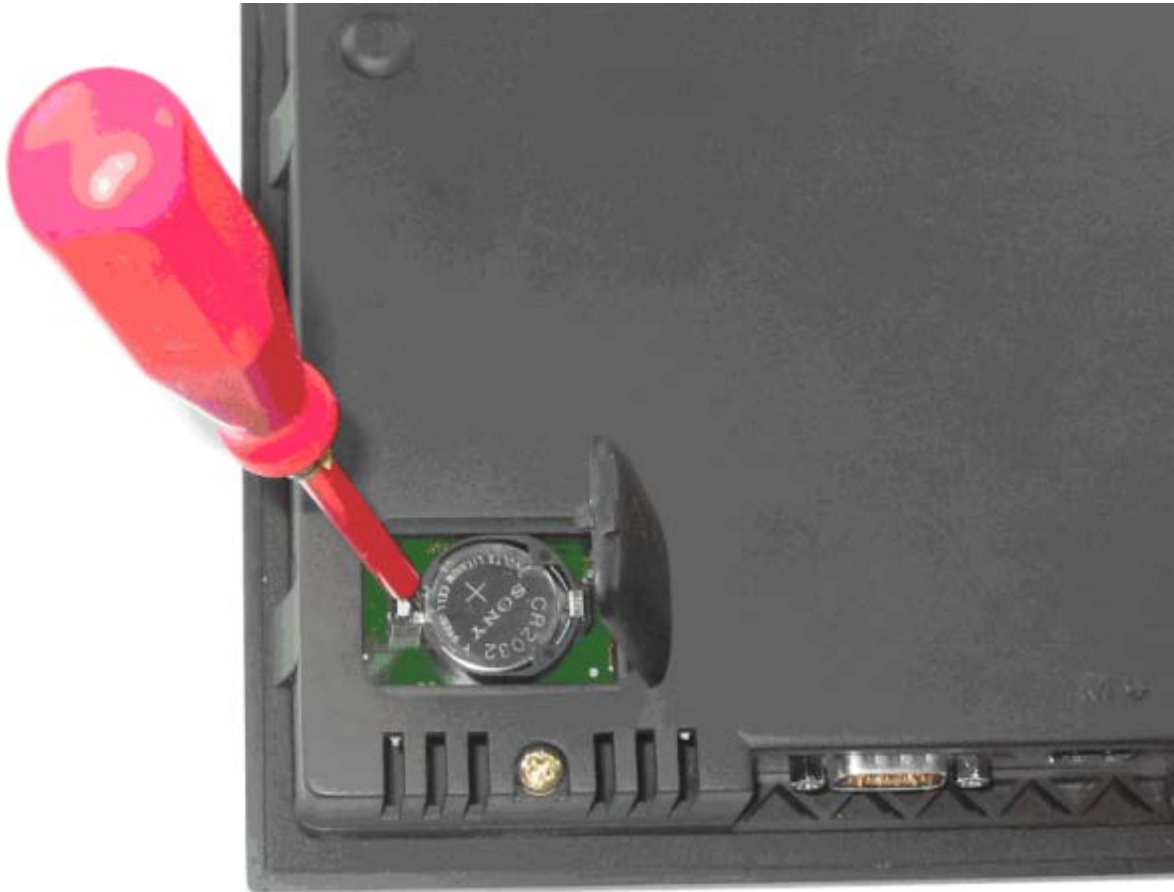
Figure 11-14 Replacing the backup battery for the cabinet operator panel
