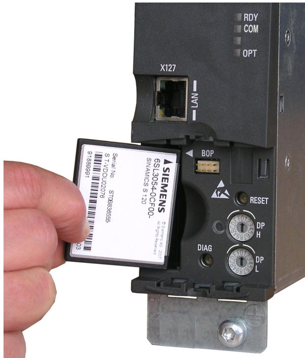
Figure 4-19 Slot for the memory card
