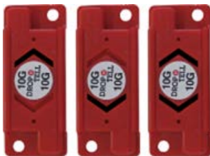
Figure 3-5 Shock indicator tripped
