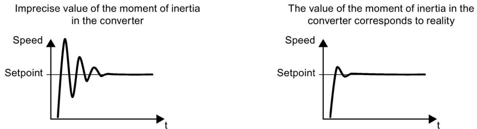
Figure 9-25 Influence of the moment of inertia estimator on the speed
