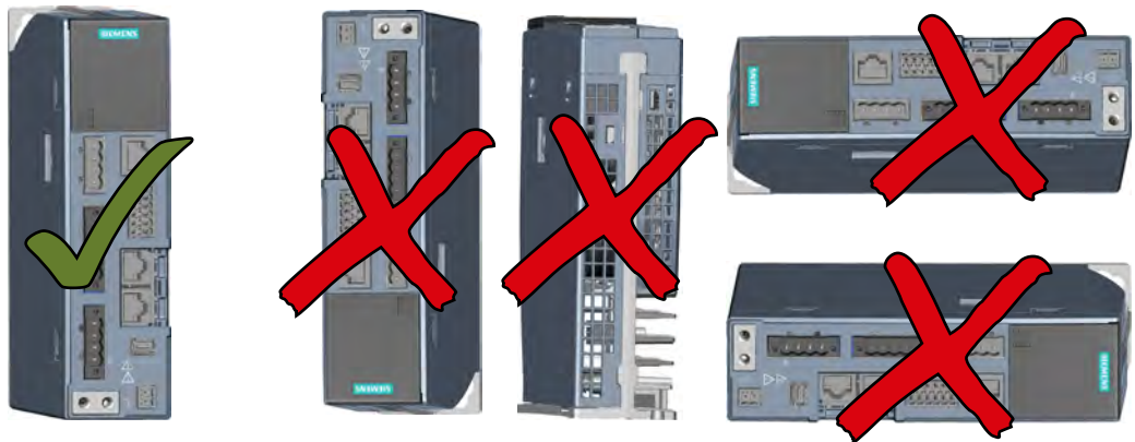
Figure 6-2 Mounting position of the converter
