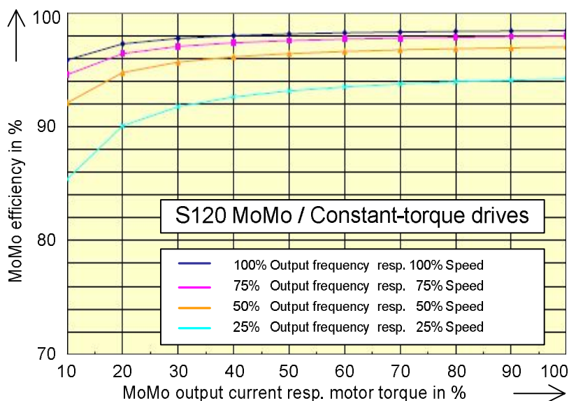
Figure 1b) Efficiency of air-cooled SINAMICS S120 Motor Modules in constant-torque drives as a function of the output current ratio in %
