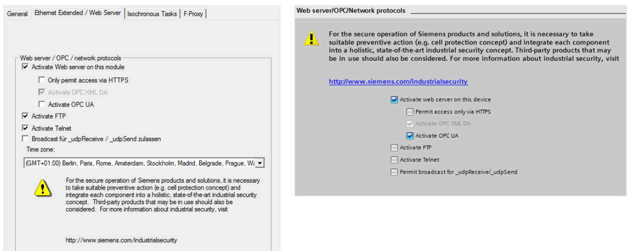
Figure 8-10 Activating the SIMOTION IT Web server functions in SIMOTION SCOUT or SIMOTION SCOUT TIA
