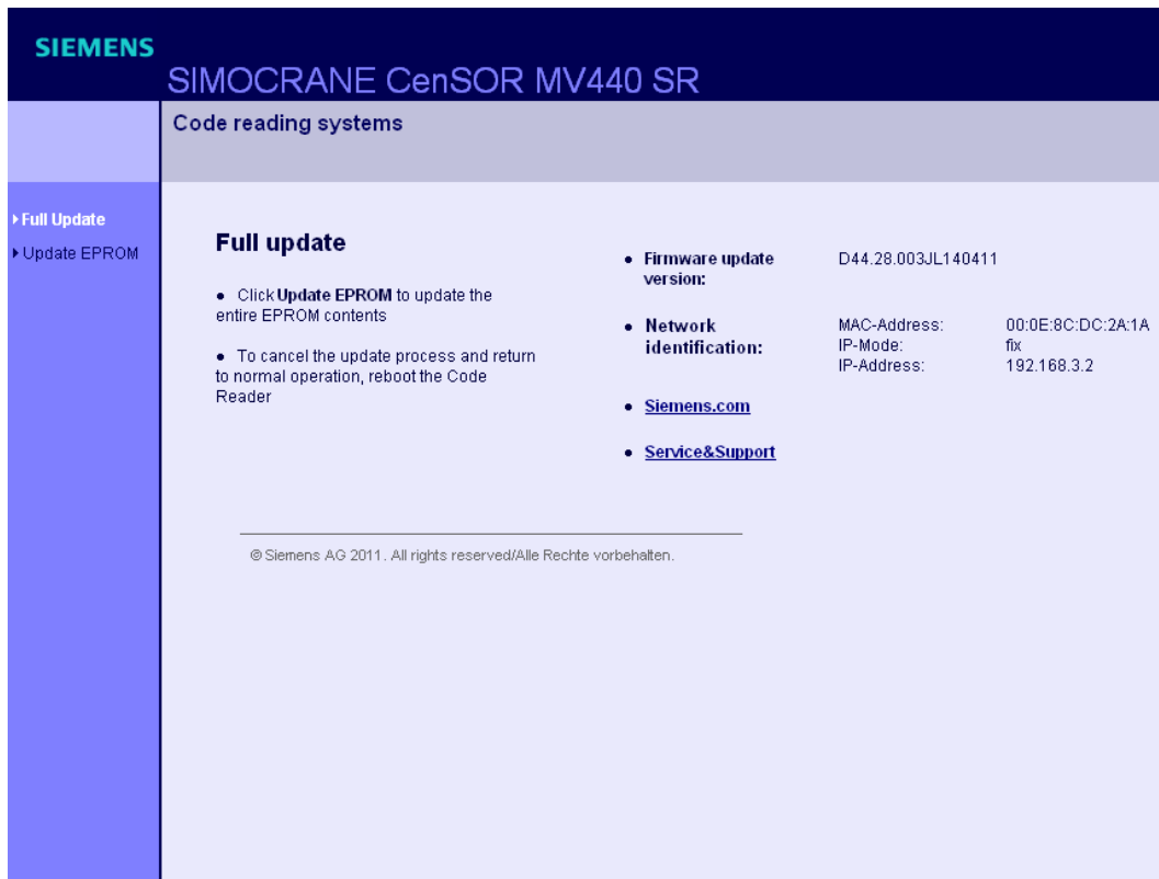
Figure 8-21 Updating the firmware of the SIMOCRANE CenSOR MV440 camera
