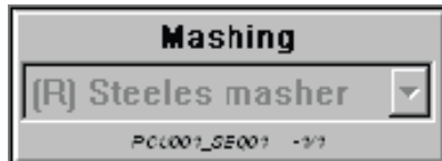
Figure 7-18 Function header of a recipe unit procedure column in the RP view of the recipe editor
