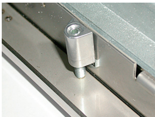
Figure 4-4 Proper positioning of the clamp
