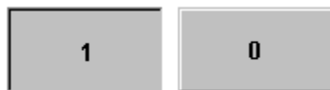
Figure 5-3 The two statuses relate to the Status button when the Switch option is set
