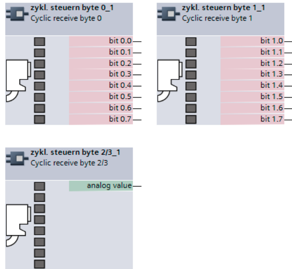
Figure 2-11 Cyclic data to SIMOCODE pro, basic type 1, 4 bytes
