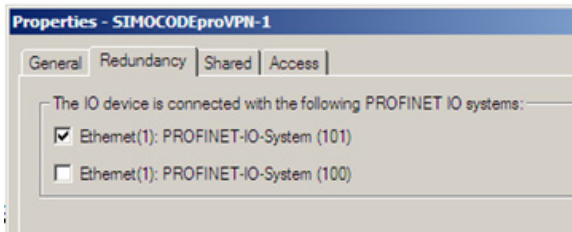
Figure 2-20 "Redundancy" tab card in module properties screen
