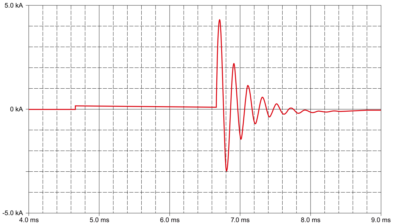
Figure 6-16 2. Energizing with a 3RT2636 capacitor contactor (with precharging) Result: The maximum inrush current peak can be reduced to less than 5 kA (depending on precharging).
