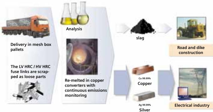
Fig. 3.8.5 – Recycling processes for LV HRC and HV HRC fuses
