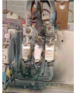
Fig. 5.8.1 – Unsuccessful disconnection of current resonance
