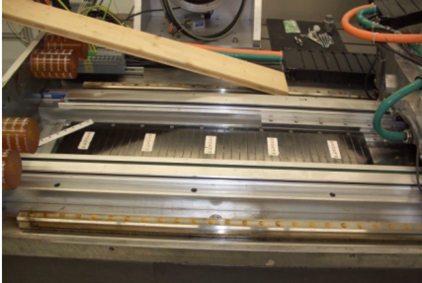
Figure 6-28 Initial situation when mounting the continuous cover band
