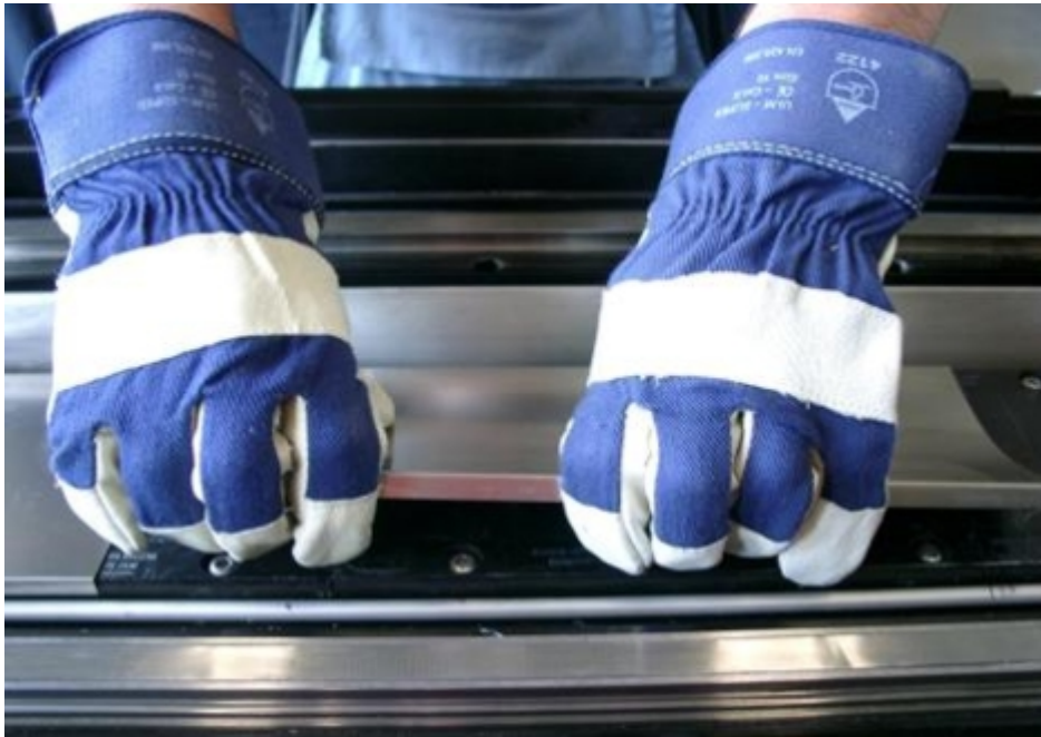
Figure 6-41 Demounting a segment of the segmented secondary section cover
