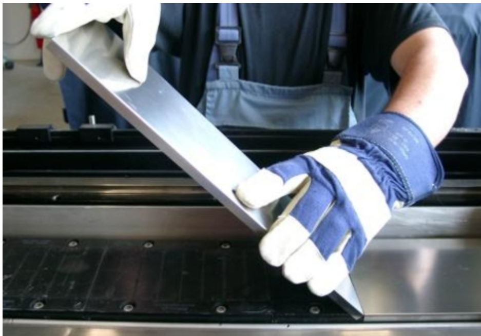
Figure 6-39 Mounting an additional segment of the segmented cover
