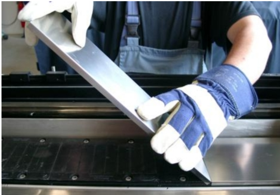
Figure 5-20 Mounting an additional segment of the segmented cover
