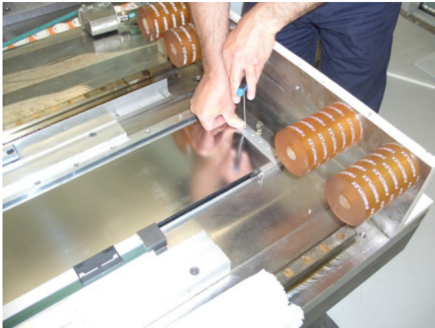
Figure 5-18 Moving up the clamping wedge
