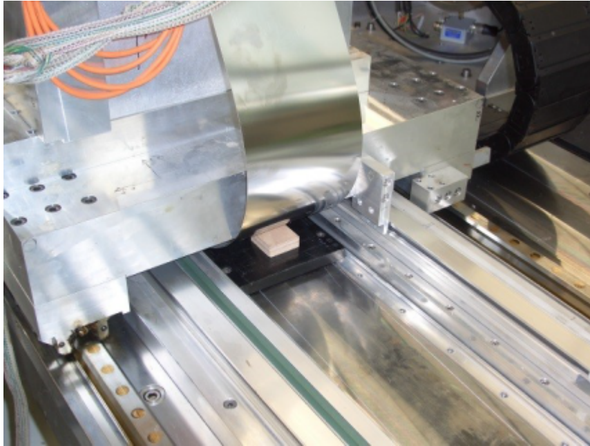
Figure 5-16 Fixing the cover band
