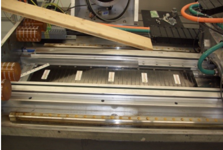
Figure 5-9 Initial situation when mounting the continuous cover band
