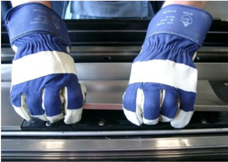
Figure 5-22 Demounting a segment of the segmented secondary section cover
