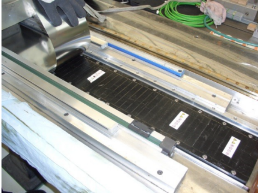
Figure 5-17 Unroll the cover band on the secondary sections
