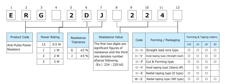
The above example shows an anti-pulse resistor, 2 W power rating, resistance value of 220 k ohms, tolerance  $\pm$ 5 %, and package of standard bulk packing.
