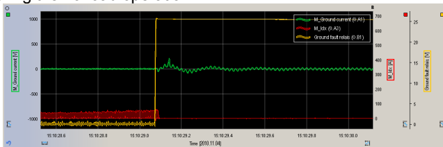
Figure 12: Earth Fault testing (LCI ASDS)
