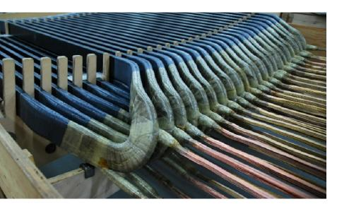
ABB's LV200, LV VPI 300s, LV400, HV VPI, and HV600 insulation systems are designed with the latest materials and processes to meet industry standards. When coupled with proven stator engineering design standards, the stator winding will provide years of trouble-free operation with minimal maintenance.
