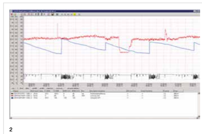
1 Visualization of the optimization objective | 2 Cleanliness per boiler section over four days | 3 User interface for graphical modeling
