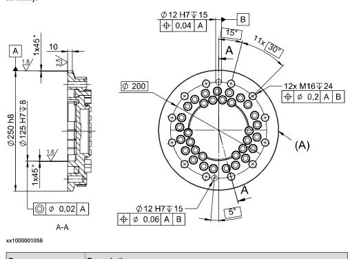
The following figure shows the robot tool flange SS-EN ISO 9409;2004 (dimensions in mm).
