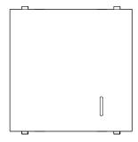
The one-channel 16A Switch Actuator is a flash-mounted device for the ABB's Mylos Building Automation system.
