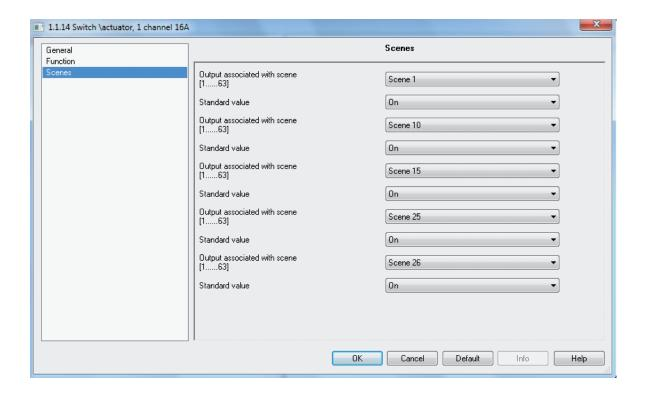
The scene function is enabled in the "Function" parameter window.
