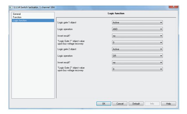
For each output the logic function makes up to two logic objects available, that are logically connected to the "Switching" communication object.
