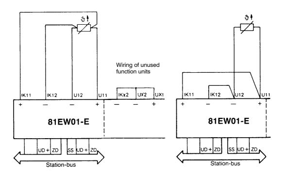
Unused function units must be bridged on connector X1 in accordance with the above connection diagram (left-hand diagram). The following applies here: X = 1...4, correspon-ding to the four function units of the module.
