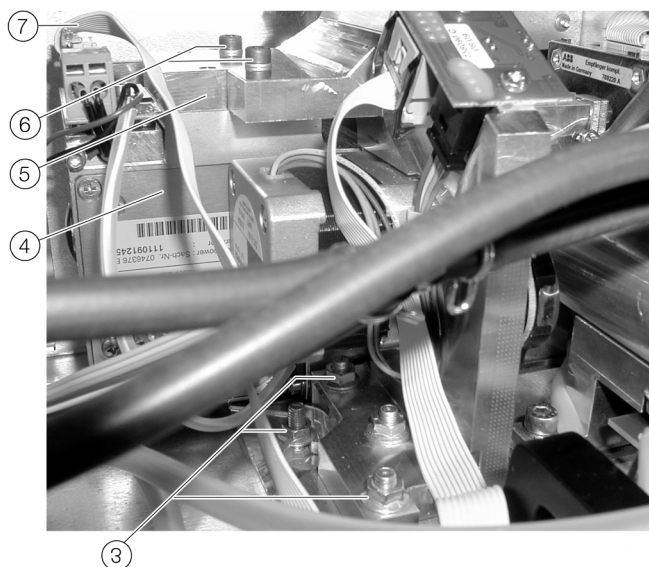
Figure 97: Removing the lamp
