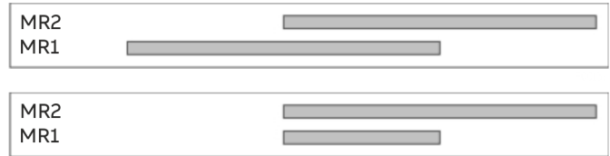
Figure 71: Two measuring ranges with suppressed zero point
