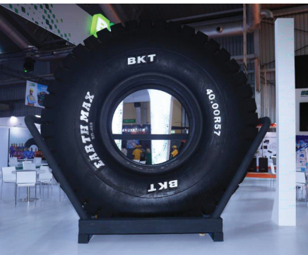
BKT's EARTHMAX SR 57 is an all steel radial tyre specially engineered for loaders, dozers and utility vehicles operating in underground mines.
