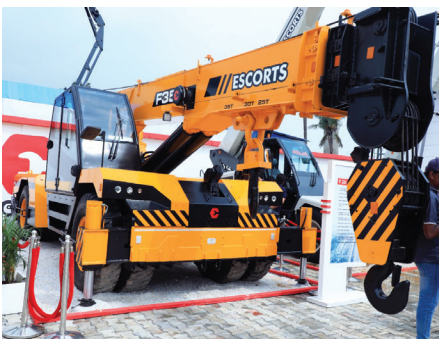
Escorts' F35 crane in 35 tonne class for the pick and carry safe segment.
