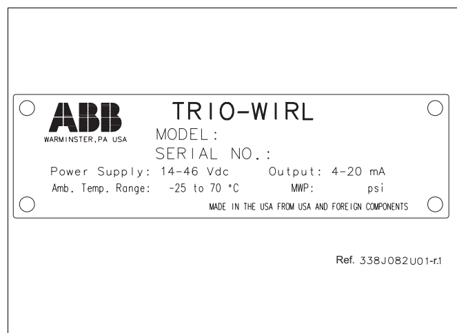
FIGURE 5-1 INSTRUMENT DATA TAG
