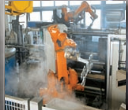
Mounted on the floor, on a shelf, tilted, inverted or on top of a machine: ABB's robot range guarantees a maximum of flexibility for die casting cells.
