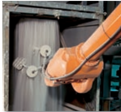
More output, less down-time: robot-based automation optimizes ceramic shell making.
