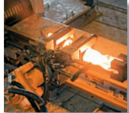
Robotized production flow in a forging operation.
