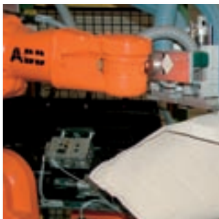
An IRB 140 robot picks up a filter from the stack.
