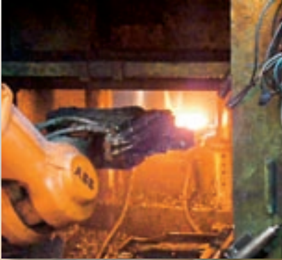
The heat is on: Forge rolling applications require heat-insulated gripping tools.
