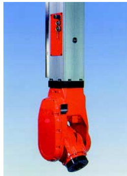
The wrist unit of the arm-type robot IRB 6400, with two rotating axes, used on the gantry robot IRB 8400/FP-5
