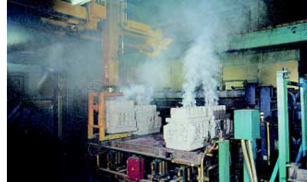
Palletizing of casted engine blocks in a foundry using an IRB 8400/FP-5
