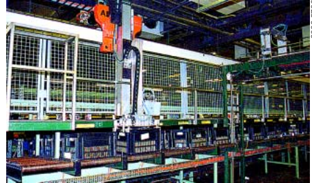
Orderpicking of milk and yoghurt in a dairy using an IRB 8400/ZP-4
