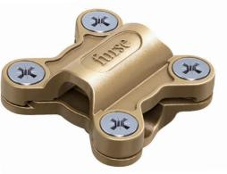
Furse® Conductor Clamps are made from high quality copper alloy, providing the perfect conductor connection within a lightning protection and earthing system. Our clamps offer solutions for both stranded cable and tape conductors.
