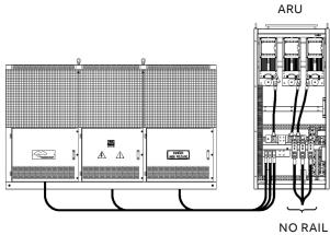
The ARU needs to only read the traction voltage and current in order to operate optimally within a new or existing traction power system.
