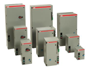
The enclosed Pro-S starters series offer a variety of models to cover the majority of applications. They're available as across the line, reversing, 2-speed 1 winding, 2-speed 2 winding and single-phase versions. All starters are offered in either a NEMA 1, 4/12 or 4X enclosure and in multiple combination with a fusible disconnect switch, non-fusible disconnect switch or circuit breaker.
