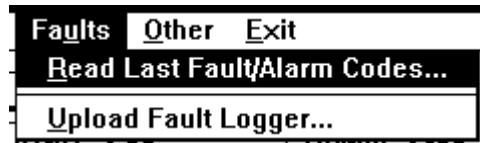
Figure 10 - 1. Pull-down menu for Faults. Note that some menu commands may be inactive if it is not possible to use them in the current situation.
