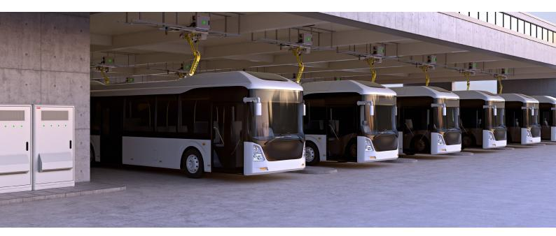
Pantograph-down depot set offers an ideal solution for charging electric buses fleet with an inverted pantograph positioned over the vehicle at depot for overnight or long charging session.
