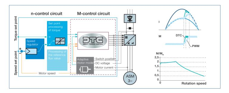
ABB's dynamic control of asynchronous and PM servo motors enables the rapid correction of load-side disturbances. ABB drives with direct torque control (DTC) provide speed and torque control without sensors.
