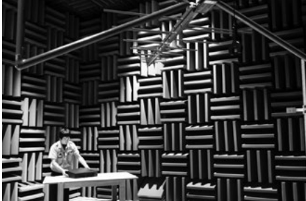
Acoustic radio wave anechoic chamber
