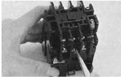
Pull out the moving contact with tweezers.
