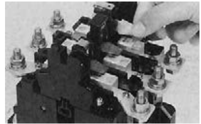
The moving contact can be removed when turned slightly. Remove the fixed contact with a screwdriver.
