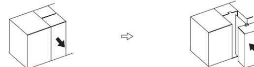
Pull forward the blank cover while push the projections located on its top and bottom.
