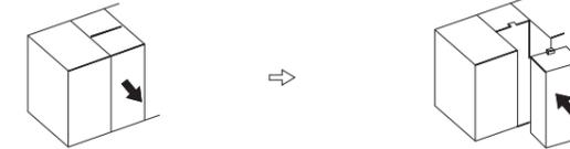
Pull forward the card while push the projections located on its top and bottom.
