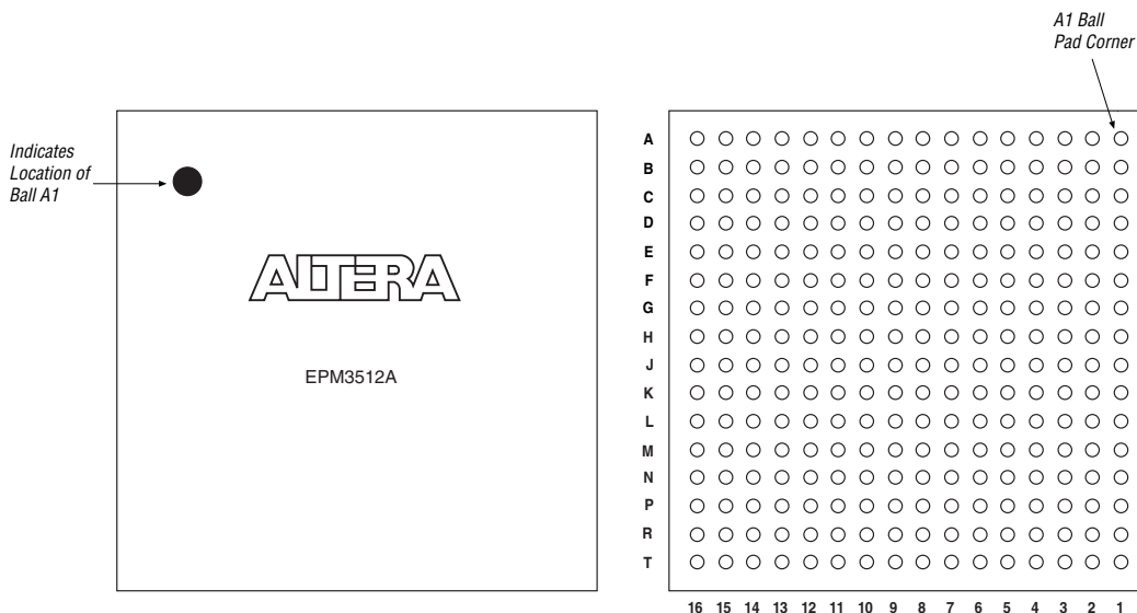
Figure 18. 256-Pin FineLine BGA Package Pin-Out Diagram
